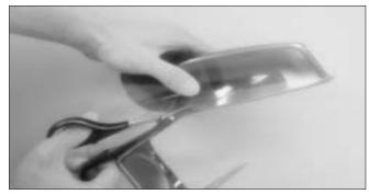
48.Locate the canopy. Cut 1.5mm(1/16") outside the molded line with curved scissors. Trial fit and trim it until it fits on the fuselage.
