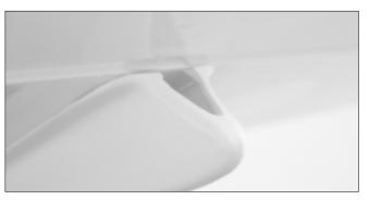
31. Enlarge the exit hole at the rear of fuselage, make sure that clevis and control horn will pass through freely.
