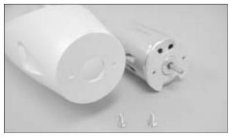
38.Trail fit the motor. When satisfied, secure the motor to the fuselage with furnished 3x5mm countersunk screw.
