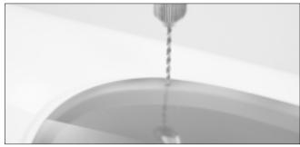
49. With the canopy in place on the fuselage, drill three holes with (1.5mm)1/16" bit. One in the front of canopy, two at both rear sides of the canopy.
