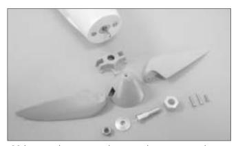
39.Locate the prop, spinner and screws as shown. Assemble the folding prop first. Make sure the two blades move freely. Insert the drive nut to the backplate then the drive shaft. The hole of drive nut is tapered to accommodate the drive shaft. Secure the whole set onto motor shaft with the nut. Do not over-tighten the nut as it might break the aluminum drive shaft but make sure it will not spin out when it in high rotation.
