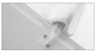
33.Thread the clevis on the pushrod (Long) then cut a small piece of silicone tube and slide it on the clevis. Insert the pushrod through the fuselage and snap the clevis on the control horn.
