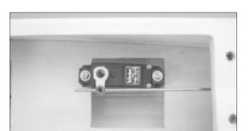
36.Insert the pushrod through the EZ connector then secure the horn on the servo when elevator in neutral position. Secure the pushrod with the 3mm set screw.
