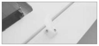
11.Install the control horn and secure it with the 2x8mm machine screw.
