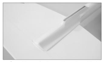
26. Spread the rear fuselage and insert the stab in the place. Make sure the tail fairing is a perfect match with the stab.
