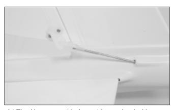
34. The kit comes with the rudder pushrod. You may choose to have rudder control by cutting the vertical fin. Trim the rudder then tape it at both side. Install the control horn and connect the furnished pushrod (short). You will have to drill a hole at rudder pushrod exit fairing for rudder pushrod pass through.
