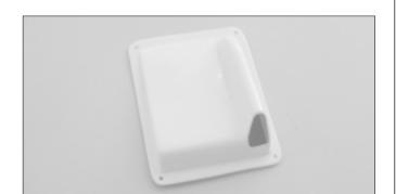
14.Locate the Hatch Cover. Cut a hole as an exit for pushrod and drill holes at each corner with 1/16" (1.6mm) drill bit, before securing the Hatch Cover, thread the pushrod rod through the exit hole.
