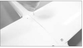
20.Place the main wing on the fuselage with the wing halves jointed CLOSELY.
