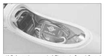
46.Refer to the manual of Electronic Speed Control Unit (ESC-50 Shown P/N: ACE8014), link to motor, battery and receiver.
