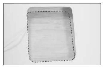
4. Glue the aileron servo tray ( square plastic piece) on the wing sheeting with instant glue.
