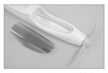
40.Make sure there is about 2mm(5/64") gap between spinner backplate and fuselage.
