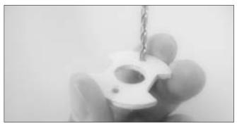
37.Locate the motor mount, drill the 3mm(1/8") holes at the pre-punched mark.
