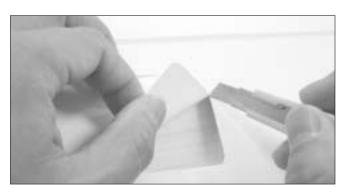
2. Cut away the covering at servo hatch and the hole near the wing root where extension wire passes through.
