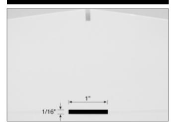
24.Cut away the covering both at the center leading and trailing edge as shown.
