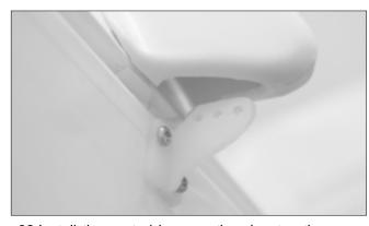
32.Install the control horn on the elevator, the same as you did on the aileron. The control horn is right after the pushrod exit hole of fuselage.
