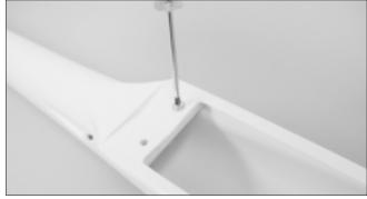
21.Remove the wing and screw the 6/32 wing bolt all the way in so the blind nut is fixed in the wing mount.
