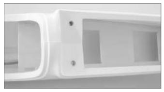
23.Locate the plywood servo tray. Insert the tray from the wing saddle opening and trial fit into the fuselage as shown. Trim the radio tray if necessary to obtain a proper fit in the fuselage. Slightly sand the inside of fuse with 200 grit sandpaper then glue the servo tray in place with epoxy or thick instant glue.
