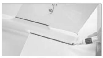
27. Trial fit the vertical tail in place. When satisfied, use pencil or marker to draw lines against the edges of fuselage.
